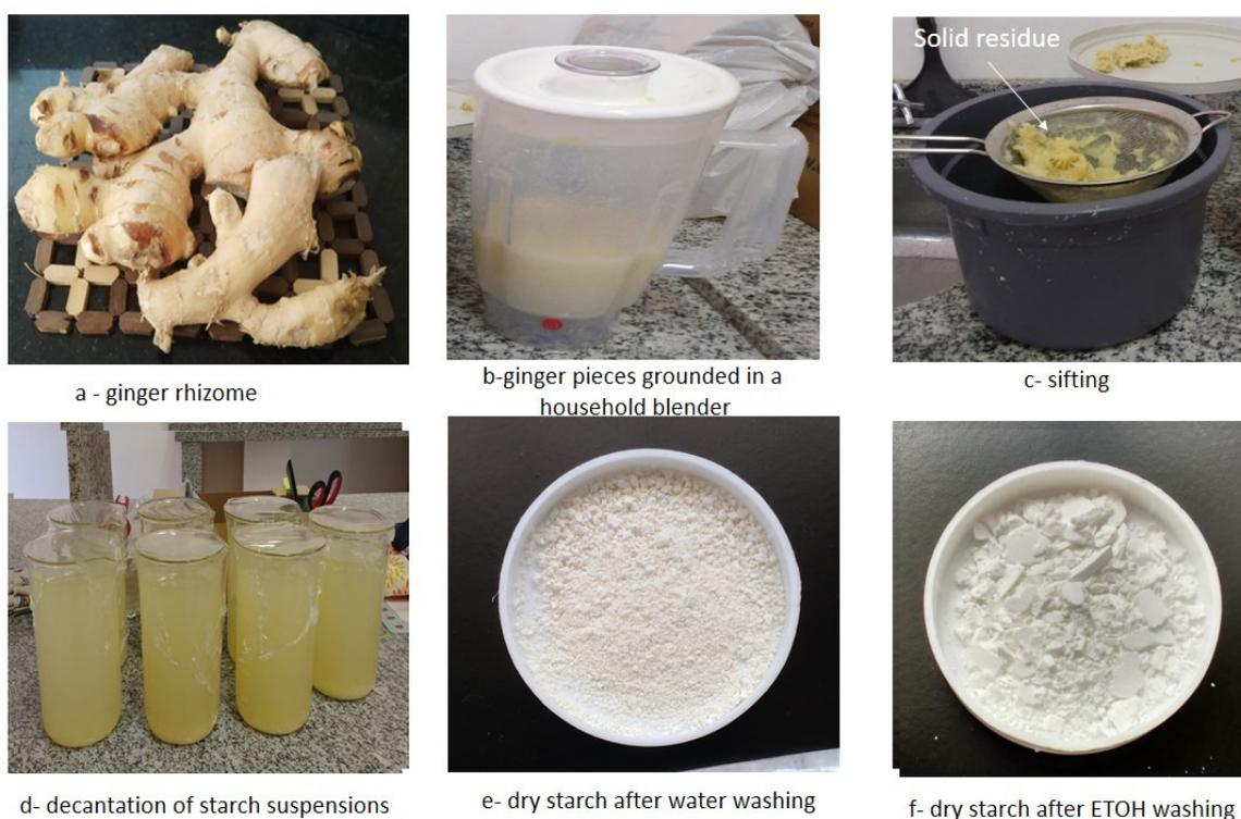
**Figure 1** - Representative scheme of the process of obtaining ginger starch from the rhizome.
