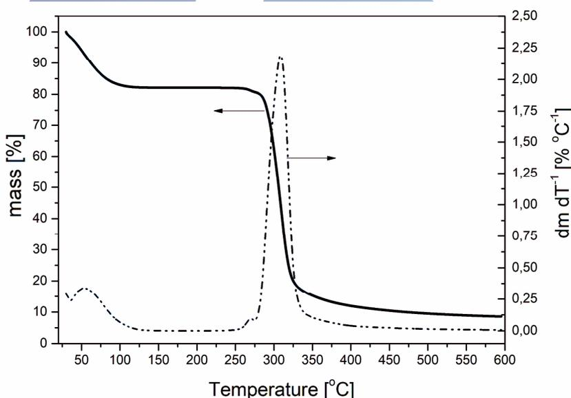
**Figure 4** - TG and DTG curves of GS. Analyses in nitrogen atmosphere, heating rate of  $10^\circ\text{C min}^{-1}$ .
