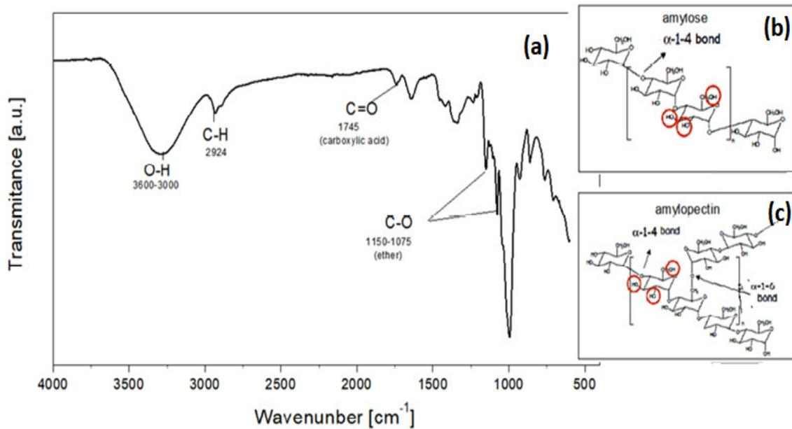
**Figure 2** - (a) IR spectrum of ginger starch (GS); (b) and (c) representative structures for the major starch components amylose and amylopectin respectively.
