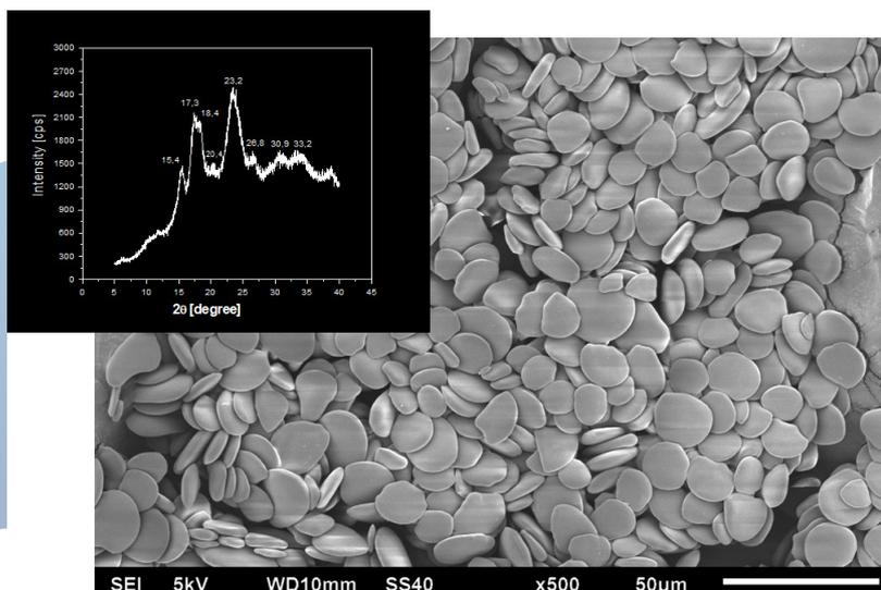
**Figure 3** - X-ray diffraction (on upper left side) and FEG-SEM micrograph for GS sample. (Scale bar:  $50 \mu\text{m}$ ).
