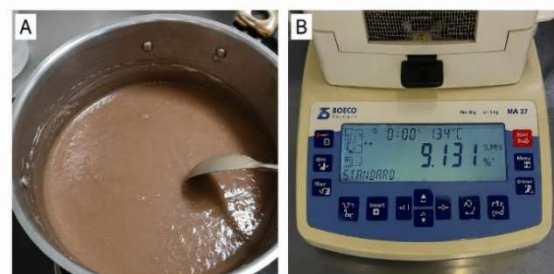
Figure 3. Pregelatinization (PGS) process: (A) starch suspension adjusted to 65% moisture content during partial gelatinization in a water bath at 75 °C for 15 min under continuous stirring; and (B) determination of the final moisture content using a moisture analyzer.
