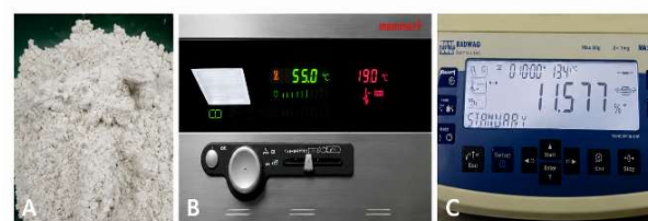
Figure 2. Annealing (ANN) process: (A) hermetic sealing of starch adjusted to 40% moisture content; (B) heat treatment in a drying oven at 55 °C for 48 h; and (C) determination of the final moisture content using a moisture analyzer.
