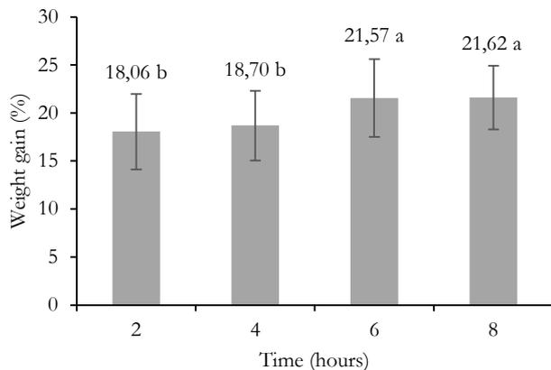
Figure 1. Weight gain percentages of *Jacaranda copaia* wood after different acetylation treatments.
